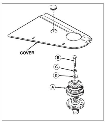
Figure 3. Install Stacked Arbor Pulley
